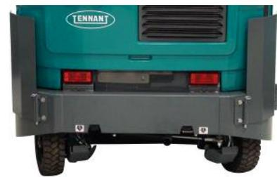
Minimize risk of damage to both the machine frame and the facility with rounded rear corners and rear tower bumpers that improve turn off from structures (walls and racking), while protecting from accidental contact.
