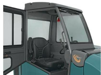
Increase safety and effective operation, in even the most severe environments, with an optional FOPS certified (ISO 3449) pressurized cabin available with heat and air conditioning.
