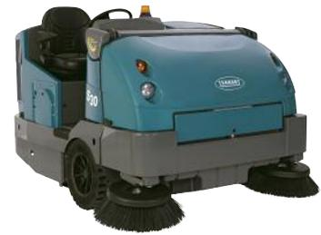
Achieve outstanding results in the harshest environments with dual side brushes which, combined with a large 14 ft<sup>3</sup> / 395 L Duramer™ hopper, allow you to sweep up to 80 in / 2,030 mm in a single pass.
